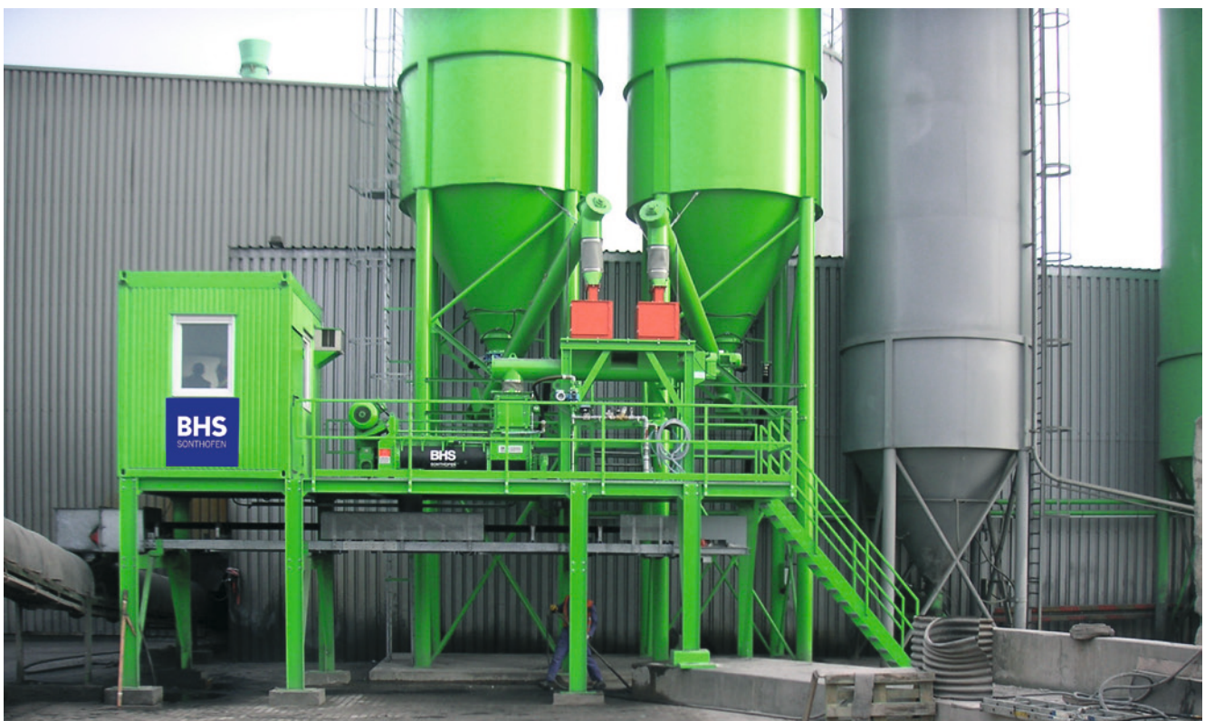
Turnkey mixing plant with an MFKG 0520 for continuous moistening of waste materials. These powdery fine materials, such as fly ash from incinerating plants, dust or fine sand, are deposited in landfills after moistening.
