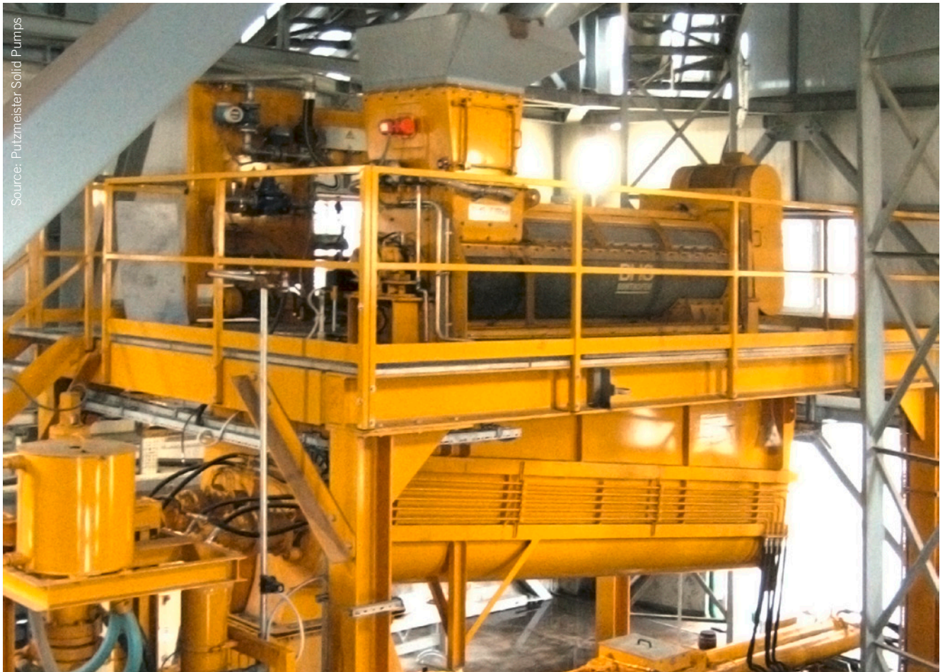
Continuous mixing plant with an MFKG 0728 for producing a suspension of fly ash and bottom ash. The mixture is then pumped into a landfill site.
