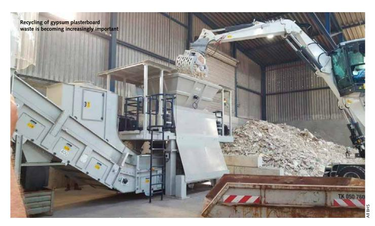
EU regulations, coal phase-out and the construction boom are among the many reasons these days for making the recycling of gypsum highly attractive. However, the process needs to be cost-efficient. BHS-Sonthofen developed a process that entails two crushing stages. This even makes it possible to recycle any adhering impurities.
