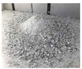
2 Gypsum waste after initial shredding in the BHS pre-shredder: The procedure allows for reliably sorting of metal parts 3 The BHS impact crusher (type PB): The combination of shredding and impact crushing produces particularly pure recycled gypsum
