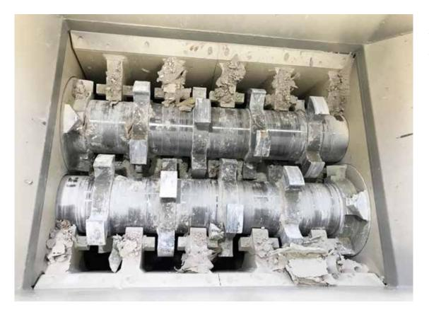
1 The two shafts of the pre-shredder of type VSR are equipped with shredding tools that can easily handle impurities in the gypsum waste
