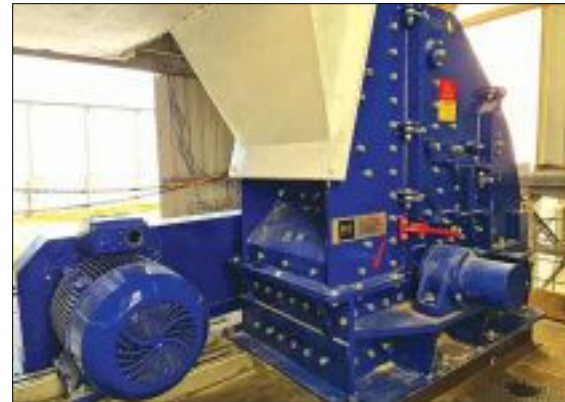
Harborlite Aegean replaced the old crusher in their plant with an impact crusher of type PB 0806 from BHS-Sonhofen.
