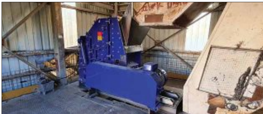
The impact crusher of type PB 0806 from BHS-Sonhofen processes two different types of perlite for the juice industry.
