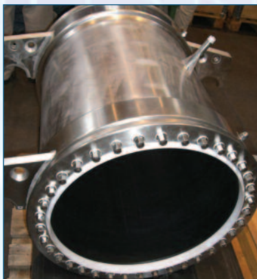
Figure 8 – Filter plate housing with membrane (shown in white).
