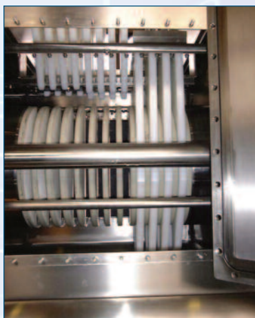
Figure 10 – Elastomeric knives sequentially and automatically discharge the circular cakes.
