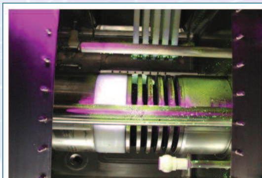
Before riboflavin test (contaminated areas are shown in green/purple)
